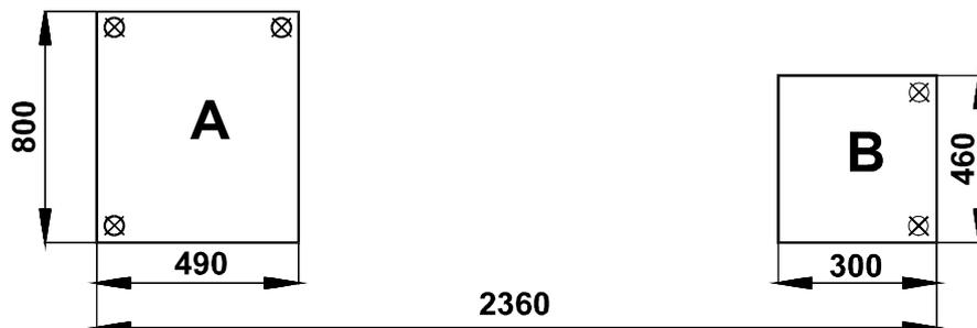
Surfaces A and B must be balanced horizontal in one surface. The winding machine is moved by lifting at 3 pendant eyes. At the winding of heavy coils there is recommended to fix the base frame with screws M 12 directly to flooring surface in marked points.
